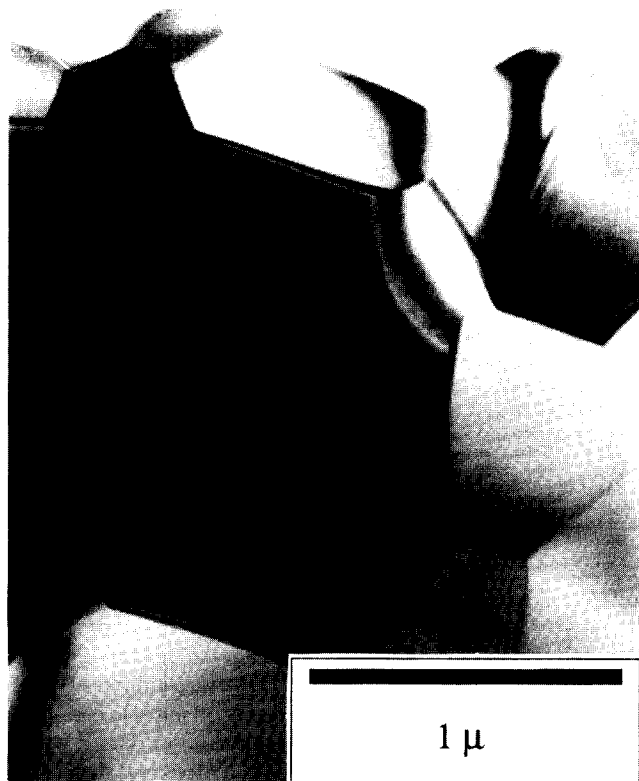
Fig. 4 Microstructure of AlN sintered at 1730 °C with 15.6 MPa for 5 min in air with no sintering additives. Note the equiaxed polycrystalline structure with no apparent porosity. The mean grain size is 0.77 \pm 0.1 \mu\text{m} .
